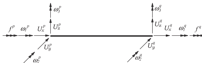
Fig. 2. Nodal displacement vector of a Hermitian beam element.
